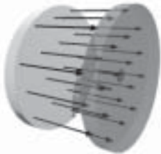
Capacitance effects the electric field between conductors
