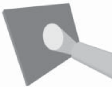
If the surface of the target is not parallel to the surface of the probe, the elongation of the electric field will introduce errors.
