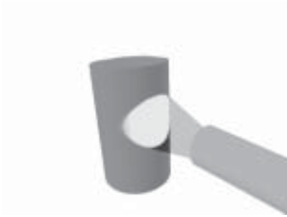
Curved targets change the shape of the electric field, affecting accuracy.
